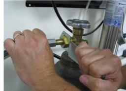
Step 3. CO2 nut should now be loosened by hand; hold the regulator body or hose (if applicable) while loosening the CO2 nut.
