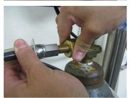
Step 4. Inspect the o-ring on the end of the tank fitting for damage. If damaged (see 2<sup>nd</sup> pic) – replace as soon as possible. If replacement is not readily available the o-ring (if not too damaged) can be flipped and reused. To flip the o-ring, the center brass retainer must be removed with a 5/16 hex key.
